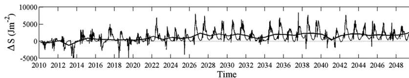
Figure 11. Difference  $\Delta S$  between the Schmidt stability of the water column simulated in the climate change scenario s5 and the reference undisturbed condition s4. A running average over 365 days has been superimposed to the daily values
