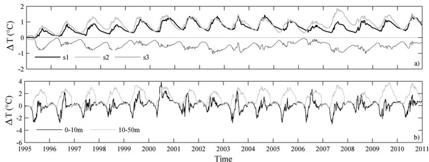
Figure 9. (a) Difference  $\Delta T$  between the volume-averaged temperature of Lake Iseo obtained from simulations without inflows and outflows (s1), with wind speed increased by 25% (s2) and decreased by 25% (s3) and the unperturbed simulation (s0). (b) Difference  $\Delta T$  between the epilimnetic (0–10 m) and mesolimnetic (10–50 m) temperature obtained from simulations with wind speed increased by 25% (s2) and the unperturbed simulation (s0)
