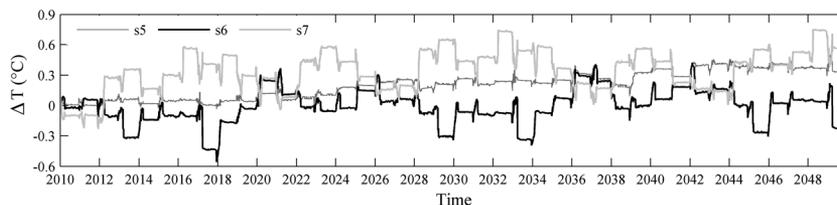
Figure 12. Difference  $\Delta T$  between the hypolimnetic (50 m–bottom) volume-averaged temperature simulated in the climate change scenarios s5–s7 and the reference undisturbed condition s4
