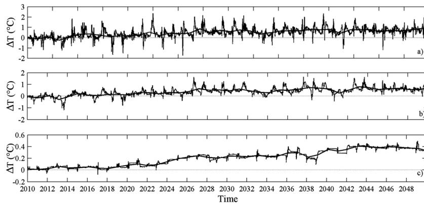
Figure 10. Difference  $\Delta T$  between the temperature simulated with climate change scenario s5 and the reference undisturbed condition s4. Temperature values have been averaged in the (a) epilimnion (0–10 m), (b) metalimnion (10–50 m) and (c) hypolimnion (50 m–bottom). A running average over 365 days has been superimposed to the daily values
