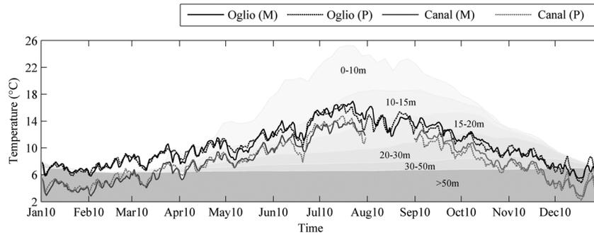
Figure 3. Comparison between the water temperature of the inflows measured (M) and predicted (P) from air temperature. The shaded areas mark the temperature range of water lying between assigned depth levels in the lake. The temperature of the Industrial Canal in August has been excluded because no volume is diverted in the Canal in this period of the year
