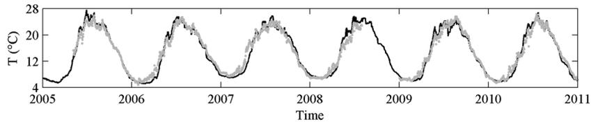
Figure 7. Comparison between simulated (black solid line) and observed (gray dots) surface (0–1 m) temperature ( $T$ ) at the exit of the Oglio River from 2005, when the monitoring of outflow temperature started
