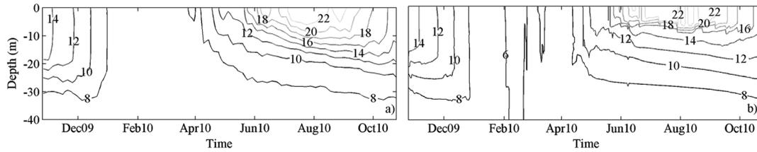
Figure 5. Contours of (a) the measured (5 days averaged) and (b) the simulated temperature field ( $CLN=5000$  and  $H_{max}=3$  m)
