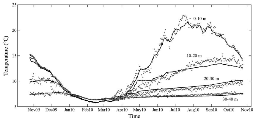
Figure 4. Comparison between the time series of the observed (dots) and simulated (continuous line) temperature, averaged over the first four layers of the water column ( $CLN = 5000$  and  $H_{\max} = 3$  m)
