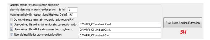
and eventually select 5H to start the extraction process. The planimetric outline of the CSs is then plotted on the screen as shown in the panel below.
